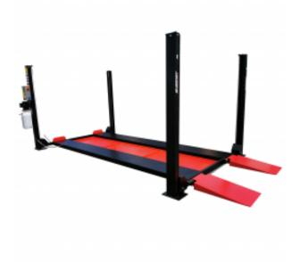
Catalog number: PK4-CARKPARK Lifting Capacity [kg]: 3700 kg Lifting height max. [mm]: 1800 mm Risinig time [s]: 44 s Power supply [V]: 400 V Engine power [kW]: 2,2 kW Type of drive: Hydraulic Synchronization: Steel rope Height [mm]: 2335 mm Width [mm]: 2850 mm Lenght [mm]: 4850 mm Weight [kg]: 820 kg
